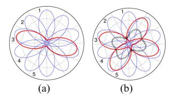
Fig. 1. Two-dimensional schema of DBFs. (a) Continuous-blue line shows the DBFs generated by an uniformly distributed tensor basis with cardinality N=5; the doted-red line shows the signal  $S(\mathbf{q})$  generated by an arbitrary DT. (b) Schema for a two fiber case, the dotted-red line shows the  $S(\mathbf{q},\tau)$  measured signals for the two arbitrary tensors, the half-addition of both signals are shown in the cross-marked black line. See text for details.
