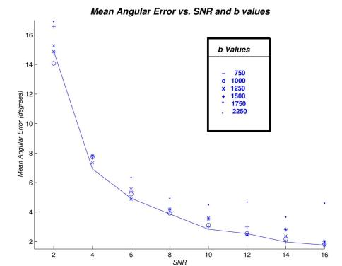
Fig. 6. Mean angular error  $\bar{\theta}$  versus SNR and b-values. M=23 diffusion measurements, tensor basis parameters  $[\lambda_1, \lambda_{2,3}, N] = [9 \times 10^{-4}, 1 \times 10^{-4}, 129]$ , diffusion parameters  $[D_{al}, D_{tr}] = [1 \times 10^{-3}, 2 \times 10^{-4}]$ , compartment sizes  $\beta_i = 1/3$ , (i = 1, 2, 3). See text for details.
