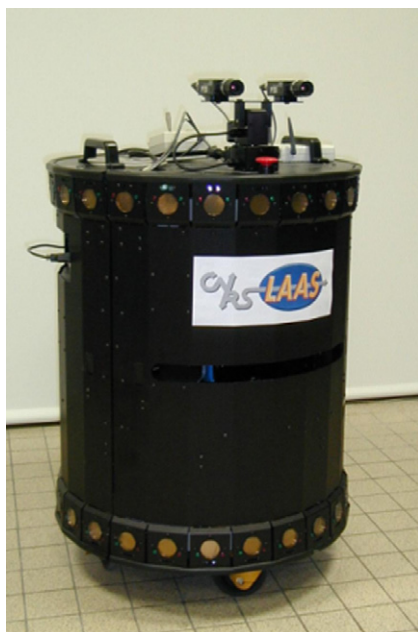
Fig. 14. The XR4000 “DILIGENT” robot we used in the experiments is equipped with a laser and BW cameras.
