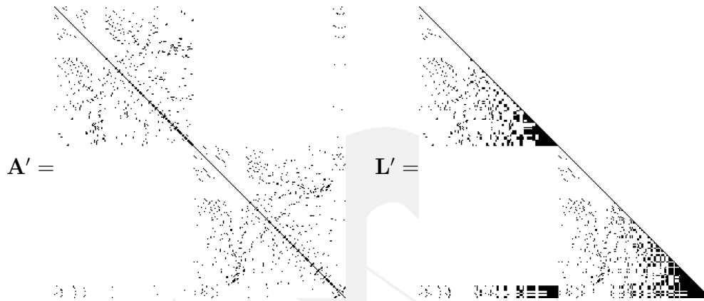
Figure 6: Representation of non-zero elements of a reordered symmetric matrix and its corresponding Cholesky factorization.
