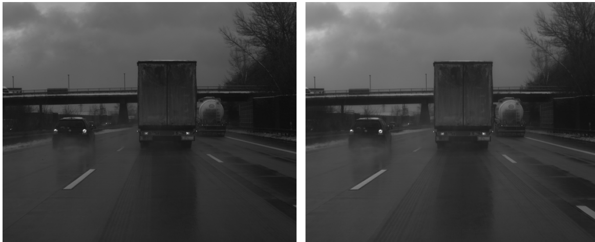
Figure 1.2: Reference frames (Left/Right) from the sequence ‘ Wet Autobahn ’ of the HCI/Bosch Vision Challenge. This sequence shows multiple adverse effects of rainy conditions. The film of water covering the street makes it reflective. Besides, the spray raised by passing cars is semitransparent, making the motion estimation on both the spray and occluded objects more complicated.
