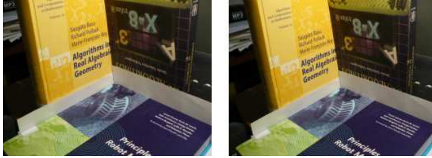
Figure 4.4: Experiment 4. Two different (but very similar) views of the same multi-planar scene. Segmentation of correspondences fails due to the type of translation movement of the camera.
