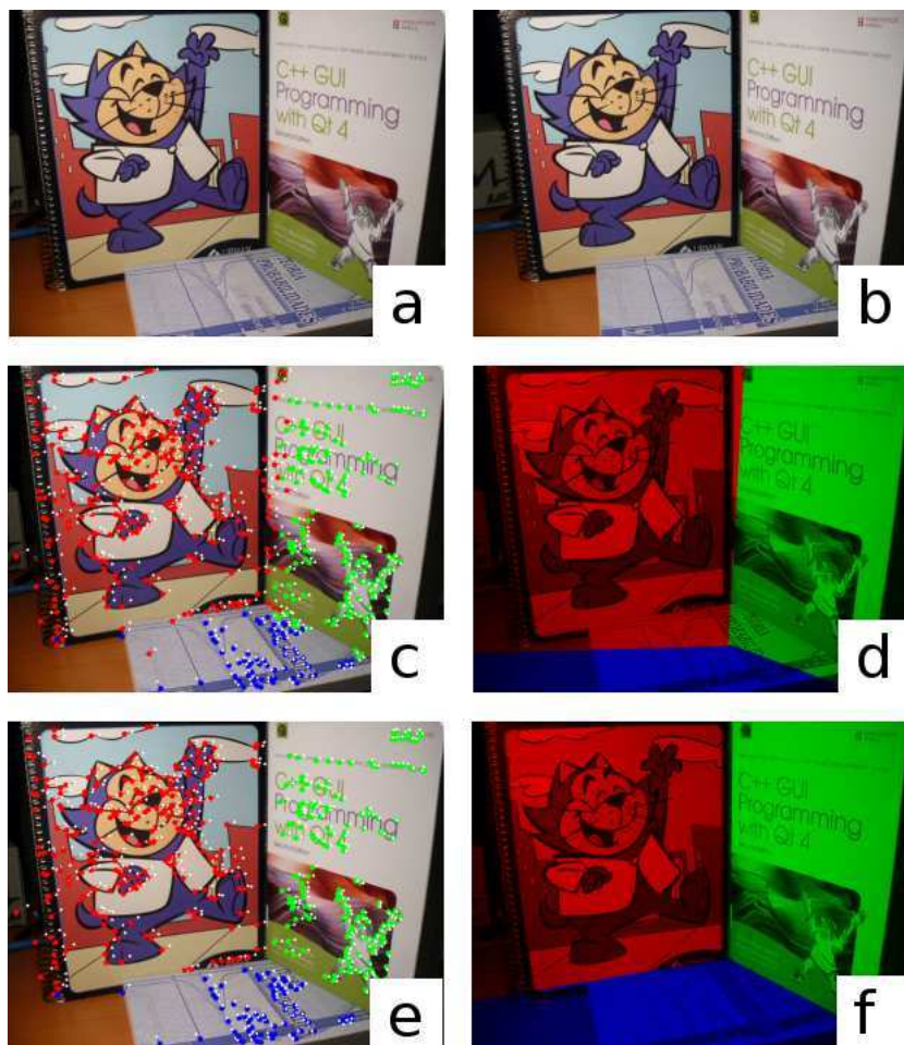
Figure 4.2: Experiment 1: Benny the Ball. (a,b) are two different views of the same multi-planar scene. (c) segmented correspondences for the detected planar surfaces. Pairs in the reference plane are red. Pairs for the second and third plane are green and blue respectively. (d) first approximation of the segmentation stage. (e) improvement of the support of each planar surface. (f) final segmentation.
