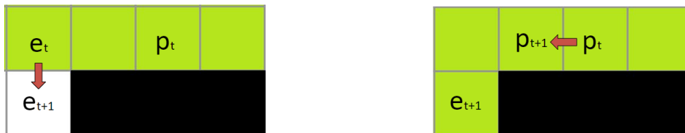
(a) In time step t + 1 the evader moves from e_t to e_{t+1} and steps out from the visibility region (in green).
