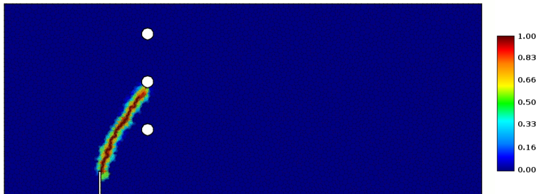
Figure 7.18: Three point bending bar with asymmetric perforations. Damage field obtained.
