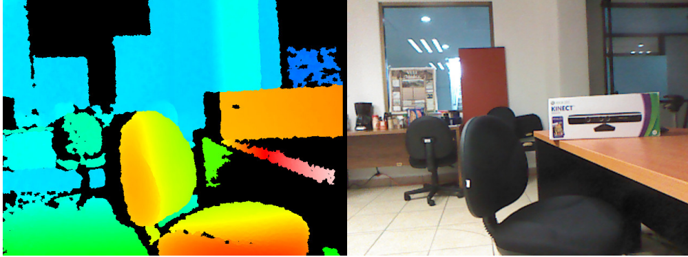
Figure 2.1: Sample data obtained with an XBox 360 Kinect. The image on the left is obtained by using an infrared sensor and a camera that triangulates depth. We present it as an intensity, here colored, where the nearest objects are red. Black regions represent blind spots, caused by out-of-range depths and reflections like on mirrors and polished surfaces. This is the case of the table, where the infrared is not perceived by the other camera.
