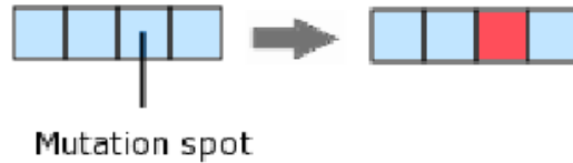
Figure 2.1: The schematic view of the simple mutation operator.
